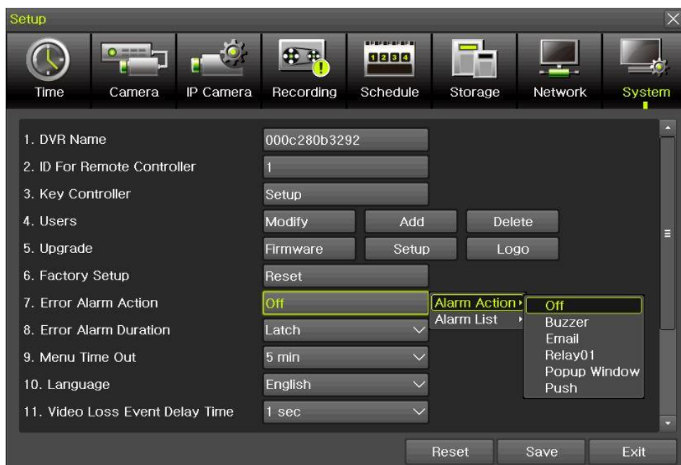
[Figure 3-48. Alarm Action]
