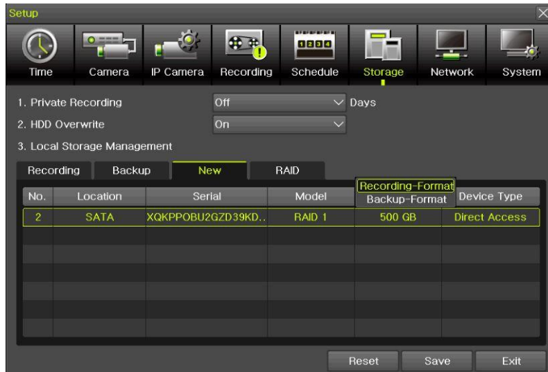
[Figure 3-35. New Storage Device Window]
