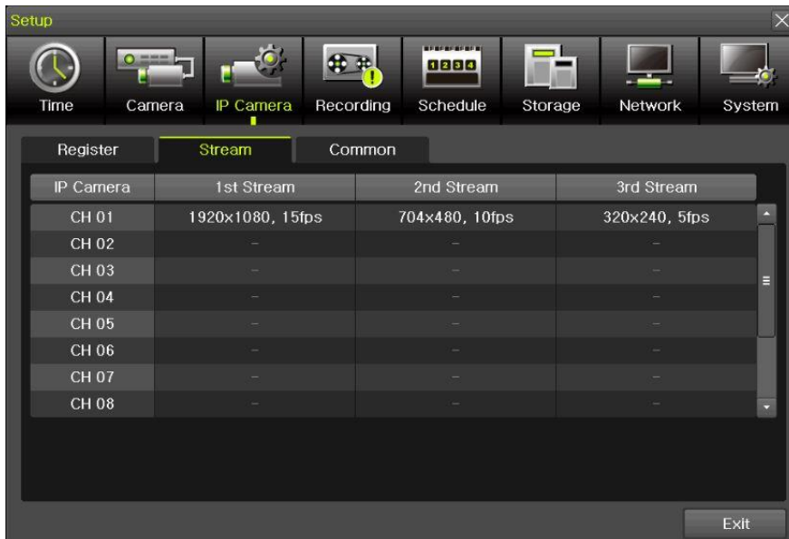
[Figure 3-19. IP Camera Stream Setup]
