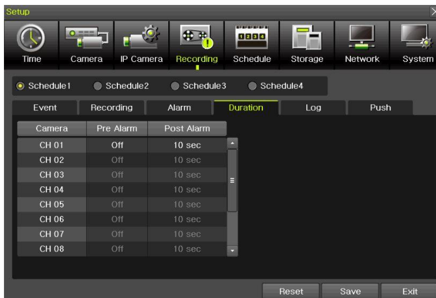
[Figure 3-28. Duration Setup Window]
