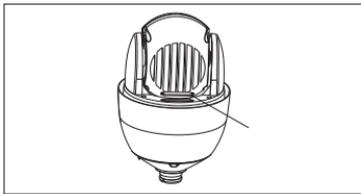
Step 3- Unscrew 2pcs screws which used to fix the transparent cover for DIP switch
