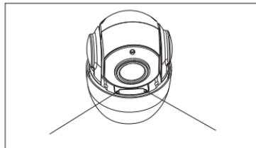
**Step 5-install transparent cover of DIP switch.**
