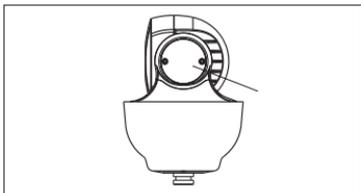
Step 3- Unscrew 2 pcs screws which used to fix the transparent cover for DIP switch
