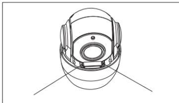
**Step 3- Unscrew 2pcs screws which used to fixed the transparent cover for DIP switch**
